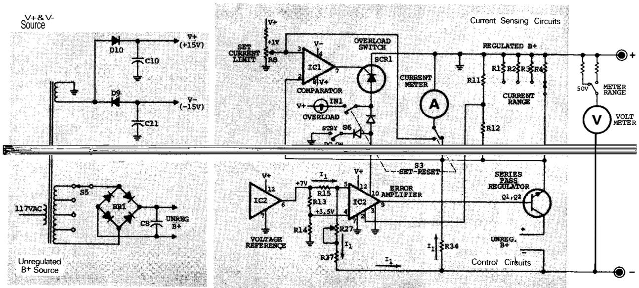
Figure 9. Power Supply Functional Diagram
