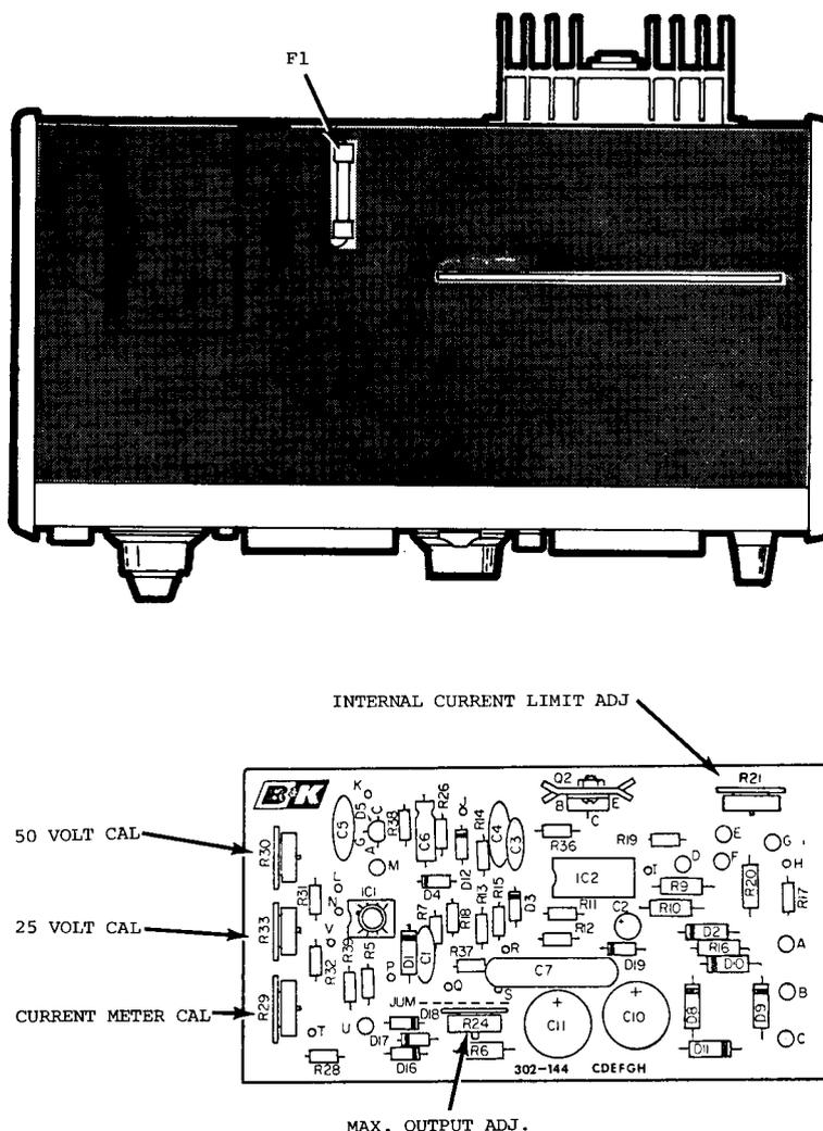
Figure 10. Location of Calibration Adjustments and Fuses
